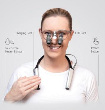
Your PowerBand is a portable control unit equipped with a rechargeable lithium-ion battery.
